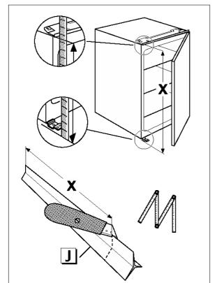
Cut the cover fillet to size and apply to the side of the cabinet.
